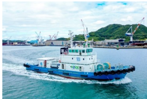
Hydrogen-fuelled tugboat Ten-Oh . Illustration reproduced by courtesy of Tsuneishi Shipbuilding Company ©.
